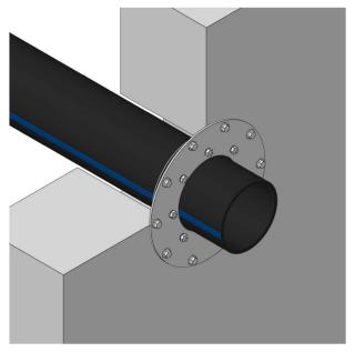
Annular space seal Hydrocord™ UKP FL-K with a special flange on one side is designed to fix the seal with fasteners to the enclosing structure. And also, for joining the seal with external waterproofing through a special butyl rubber tape.
