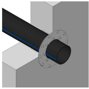
Annular space seal Hydrocord™ UKP FL-K with a special flange on one side is designed to fix the seal with fasteners to the enclosing structure. And also, for joining the seal with external waterproofing through a special butyl caoutchouc tape.
